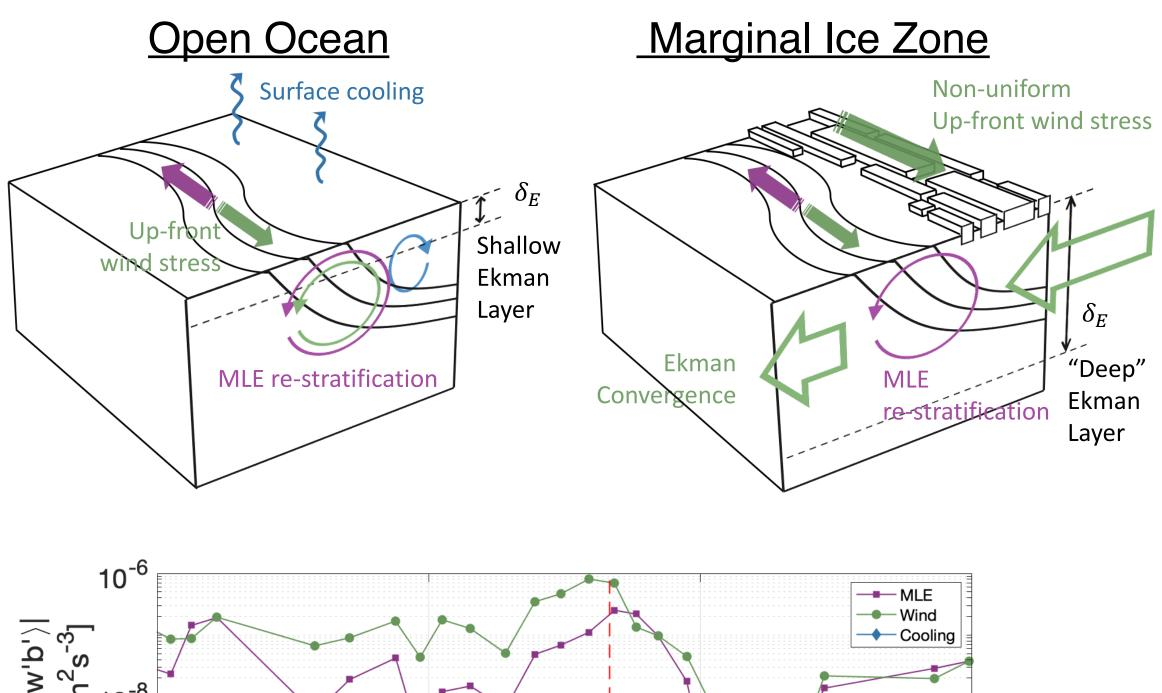
Sea ice modifies wind stress by changing the drag coefficient. There is a local maximum of stress in the MIZ. The Nonuniform wind stress causes convergence of the Ekman transport across the full depth of the front.
